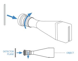
Rotate the focusing bush **clockwise** to move the lenses closer to the detector and focus objects positioned further away from the optics.
