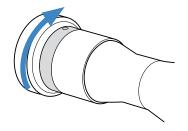
Once you have achieved the best focus position, rotate the locking ring **counter-clockwise** to lock the focusing bush.
