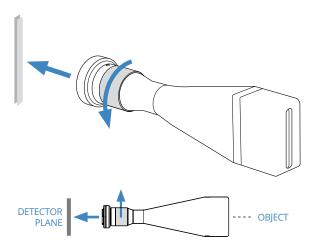
Rotate the focusing bush  ${\bf counter-clockwise}$  to move the lenses away from the detector and focus objects positioned closer to the optics.
