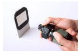
Mount the lens to a secure fixture by means of the threaded holes. Once the lens is mounted, adjust the focus until the image at the centre of the detector is sharp; you don't need to tilt the detector yet.
