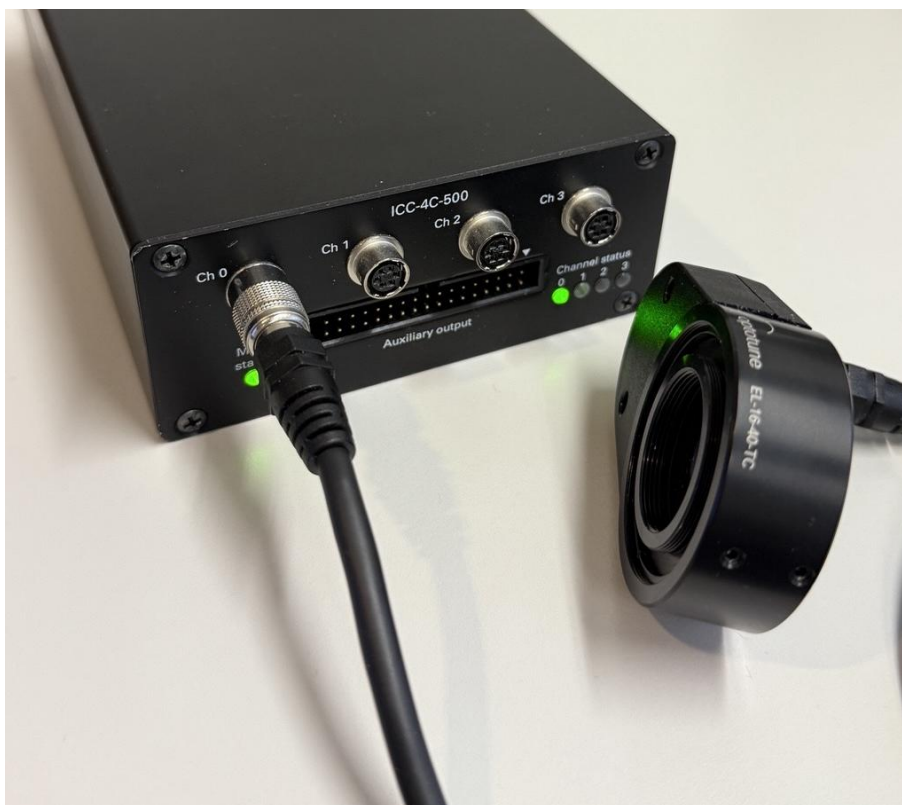
Figure 3: Connecting to a lens with Hirose connector
