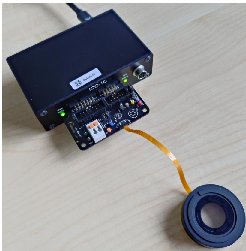
Figure 6: Connecting to a lens with FPC connector
