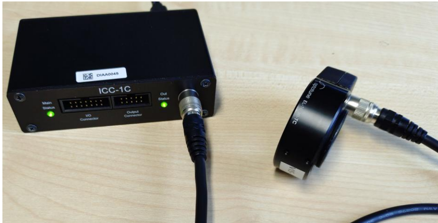
Figure 5: Connecting to a lens with Hirose connector
