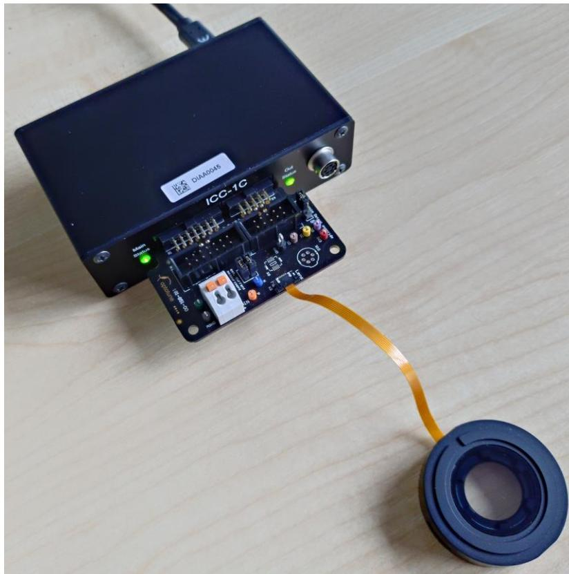
Figure 6: Connecting to a lens with FPC connector
