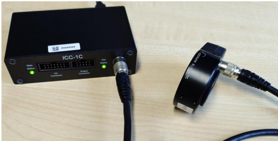
Figure 5: Connecting to a lens with Hirose connector
