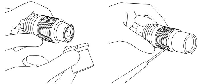
**4** Insert back in place the C-mount adaptor and fix it by tightening the socket head set-screws with an M1.5 Allen key
