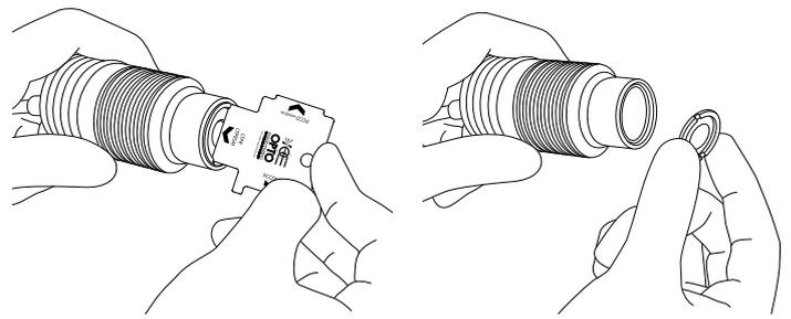
**2** Remove the retaining ring using the provided PTTOOL instrument.
