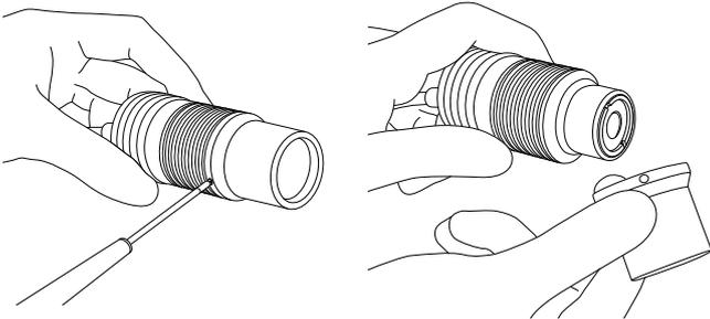
**1** Loosen the socket head set-screws by means of an M1.5 or M2 Allen key and remove the C-mount adaptor
