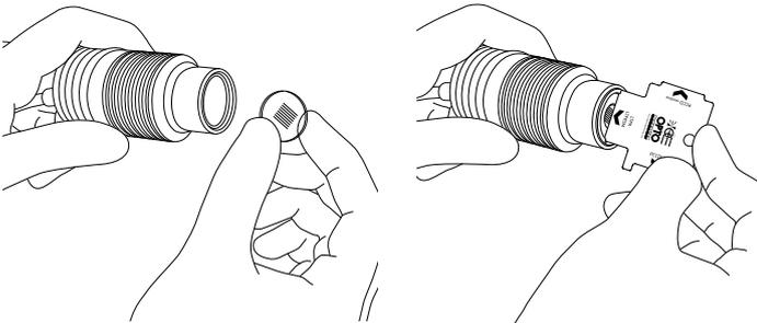
**3** Fix the projection pattern in place by screwing the retaining ring with the provided PTTOOL.
