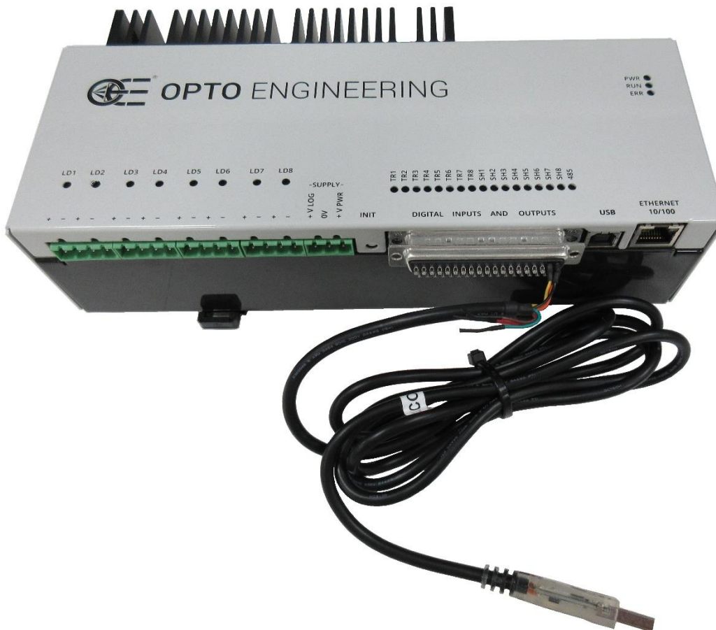
Figure 28: connection of RS485-USB adapter to the controller
