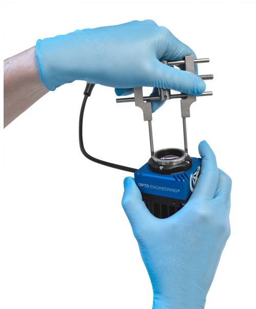
Figure 10: After removing the mount, remove the Inox steel ring.
