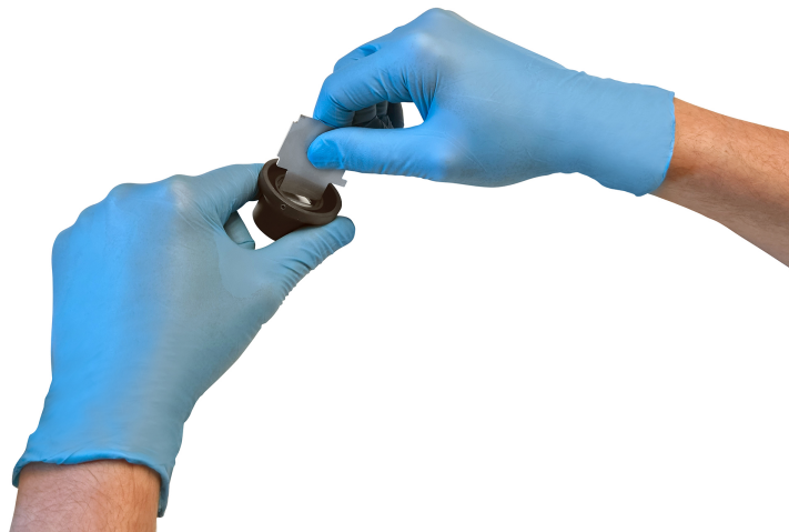
Figure 8: Second step: release the mount ring.
