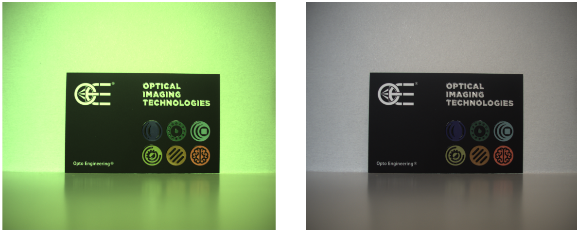
Figure 39: On the left side an uncorrected image is displayed; on the right side a white balance corrected picture is shown.
