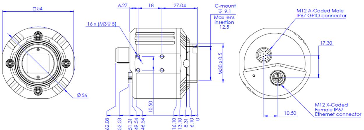
Figure 37: ITALA G.IP dimensional drawings.
