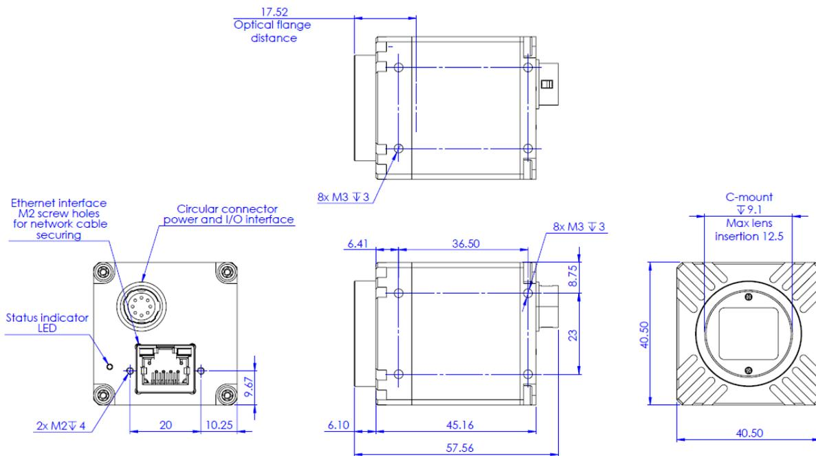
Figure 35: TYPE 1 dimensional drawings.
