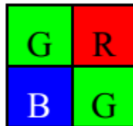
Figure 3-3 Bayer GR Pixel Pattern
