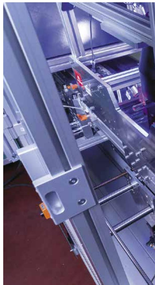
**Isotronic's VialChecker multi-camera quality control machine**
