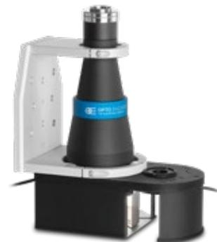
The lack of perspective given by the telecentric view of TCCAGE provides a quick alignment check regardless of the part orientation.
