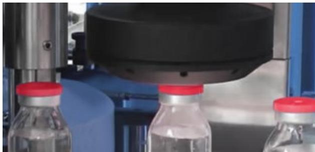
High speeds can be reached thanks to the low F/# of the PCCD lens.
