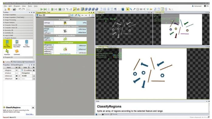
In this application, we need to sort nails amongst nuts and bolts. The image is thresholded and the resulting regions are split into blobs; finally, the blobs are classified by their elongation and the nails are easily found.
