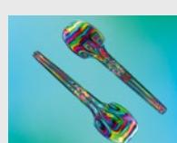
False-color image in HSV space showing the angle of polarization of plastic parts.
