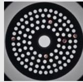
Identification of machining debris within holes through blob extraction.
