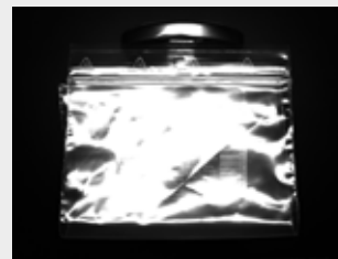
Figure 10: Polarizer placed in front of the camera to reduce reflections and improve visibility.
