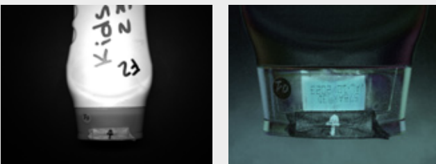
Figure 11: Reading embossed lettering. On the right, an image taken with unpolarized light, while on the left, a study in polarization is conducted.
