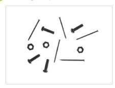
2 The image is thresholded into a region (a run-length encoded binary image) and then split into connected components.
